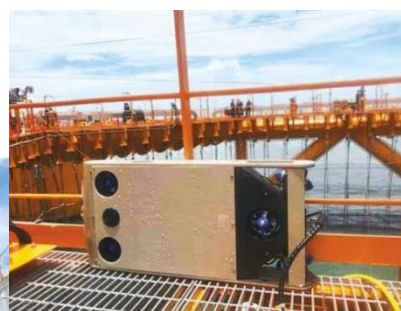
↑ Underwater robots used for inspecting underwater structures
